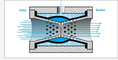
Unlike the design of conventional control valves, the sleeve and perforated cone assembly of the SF10V can maintain consistent pressure while letting process fluids from the separator pass through the valve.
